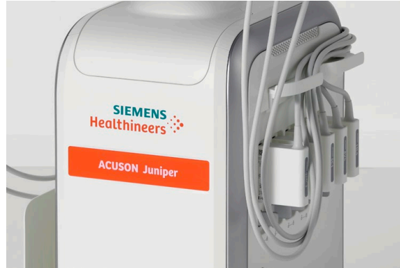
Purposeful cable management hooks – several hooks available for a clean, cable free environment.
